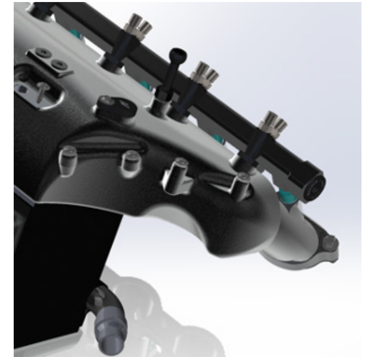
Figure 10: The Mishimoto intake manifold has a cutout area for the oil filter housing.
