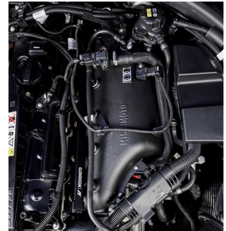
Figure 11: Mishimoto prototype intake manifold installed in a G80 M3. All the brackets and features of the factory manifold are incorporated for an easy installation and great fit and finish.
