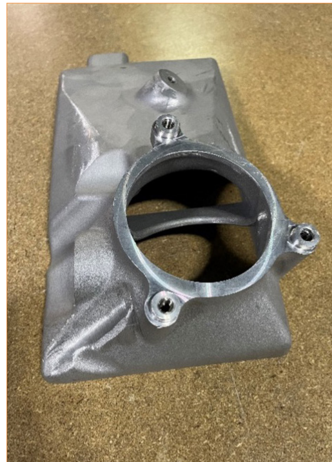
Figure 8: Intercooler Inlet with diverter
