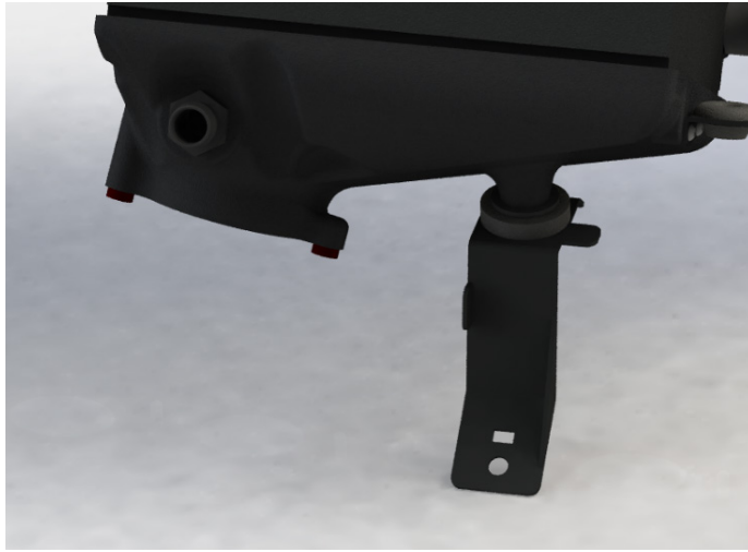
Figure 12: CAD rendering showing redesigned lower manifold mount to allow a larger, better flowing lower plenum section.
