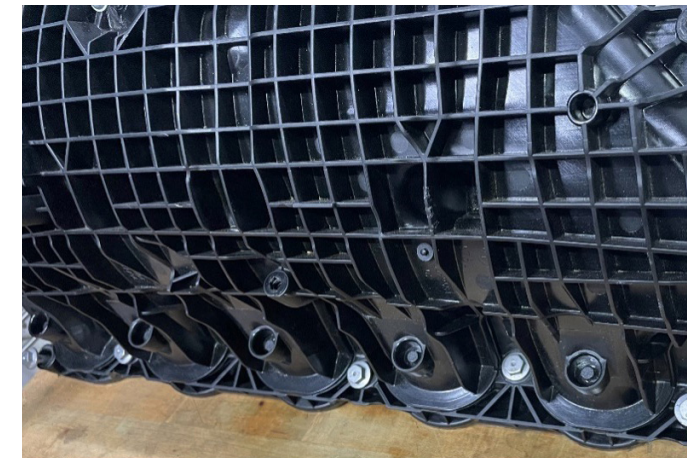
Figure 15: The factory manifold is ready to modify for adding port fuel injection.
